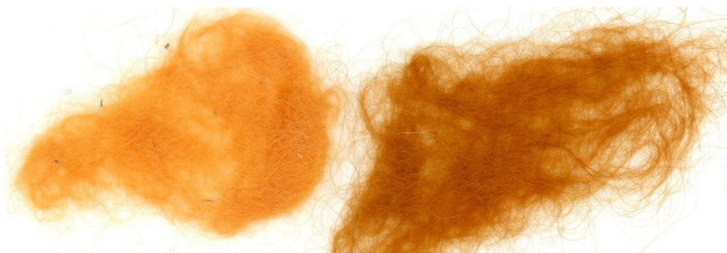
Left: White hair dyed for 12 hours with 98% pure lawsone; Right: henna with 1.5% lawsone. Application done October 30, 2018 and scanned December 30, 2018
